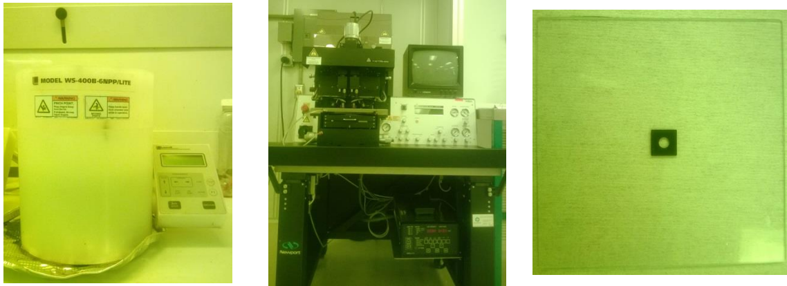
(a) (b) (c) Figure 3-5: (a) Spin coater; (b) MA6 mask aligner; (c) Photo-mask
