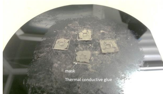
Figure 3-7: Configuration of sapphire wafers and masks for RIE
