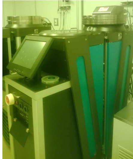
Figure 3-6: Trion MiniLock reactive ion etching system
