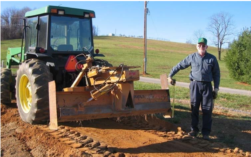
Figure 19. Topsoil scraper fabricated by Jerry Stump for leveling and removing excess topsoil above 10 cm.
