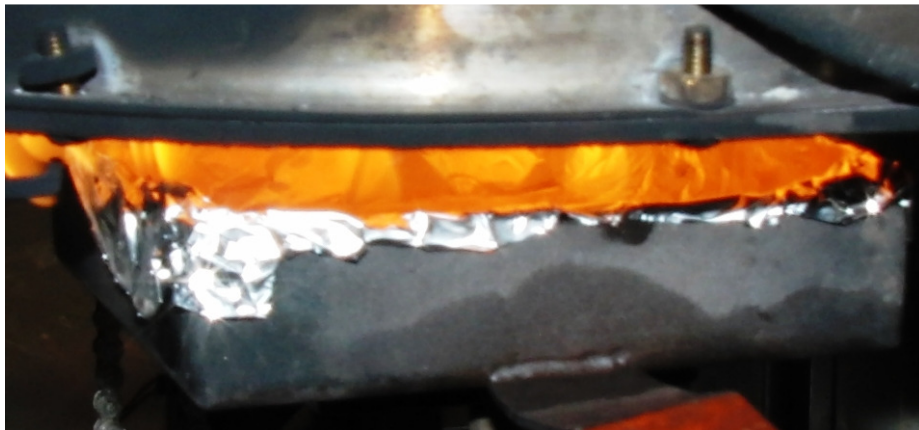
Figure 25. P184 pool fire during cone calorimeter testing.
