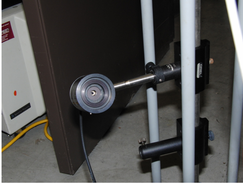
Figure 52. Photo diode for recognizing laser impulses. Upon recognizing the laser signal, the diode sends a signal to the circuit.
