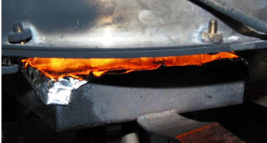
Figure 26. P117 pool fire during cone calorimeter testing.
