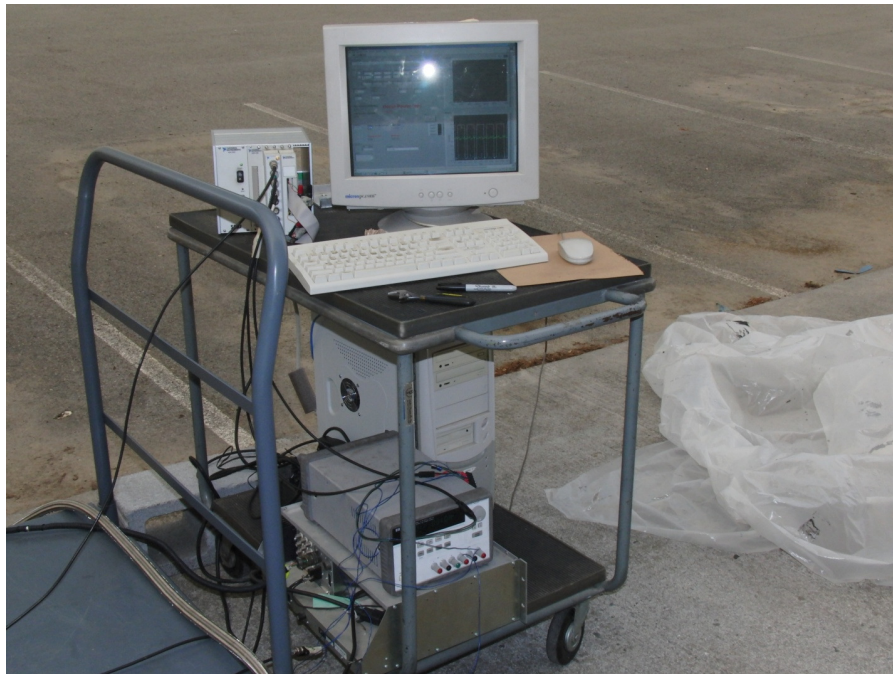
Figure 42. Data acquisition system for engine testing.
