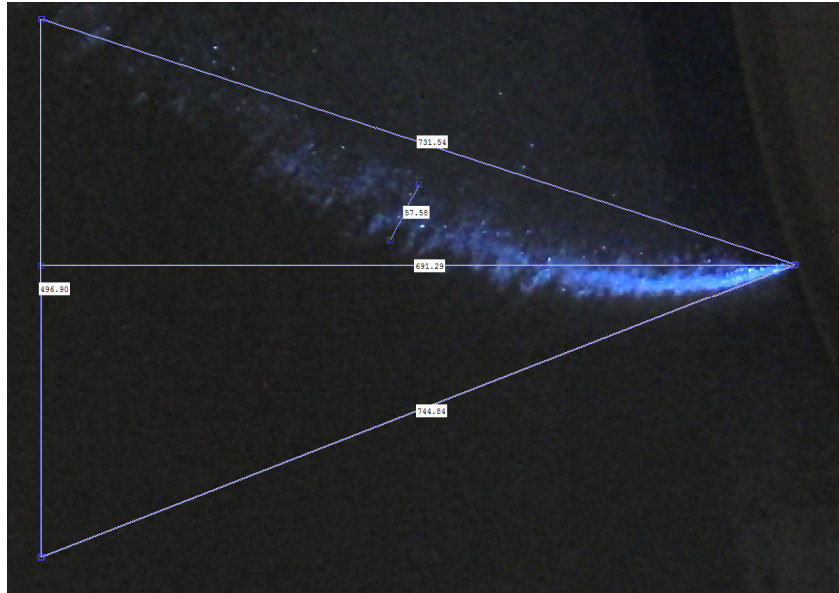
Figure 90. Jet A image processing to determine spray angle.
