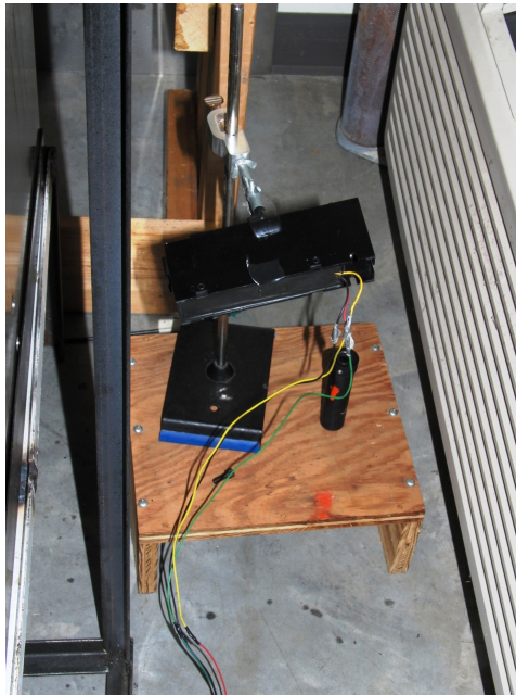
Figure 53. Laser for timing circuit.
