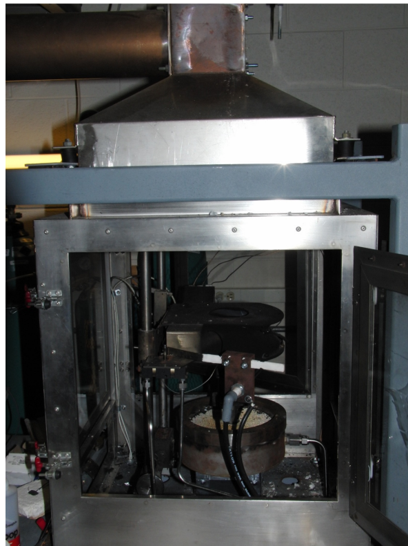
Figure 16. Combustion chamber of the cone calorimeter.
