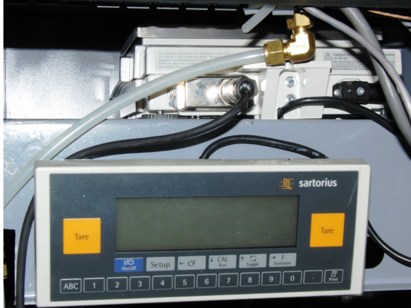
Figure 19. Sartorius load cell used to monitor the fuel mass during each test.
