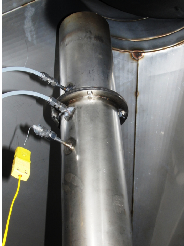
Figure 18. Orifice plate in the exhaust pipe of the cone calorimeter.
