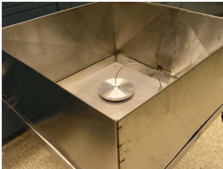
Figure 47. Original Atomizer design with shield [17] (under fair use, 2010).
