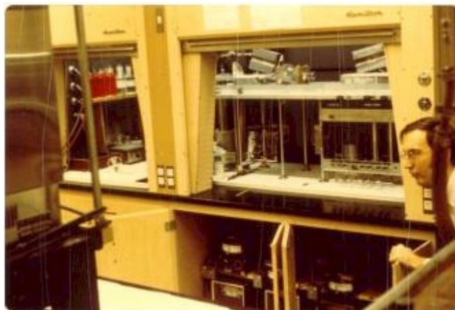
Figure 10 – Herb Maruska’s HVPE reactor where the first single crystal GaN sample was created [21].
