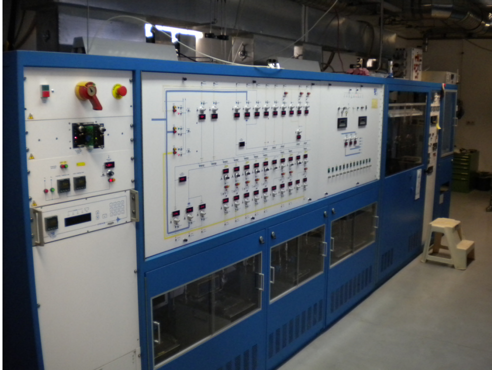
Figure 12 – Thomas Swann MOCVD reactor in the electrical engineering department at TU-Darmstadt
