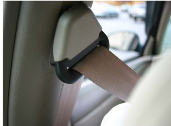
Figure 7. Directionality of the Seat Belt Webbing through the D-ring when Belt is Properly Worn
