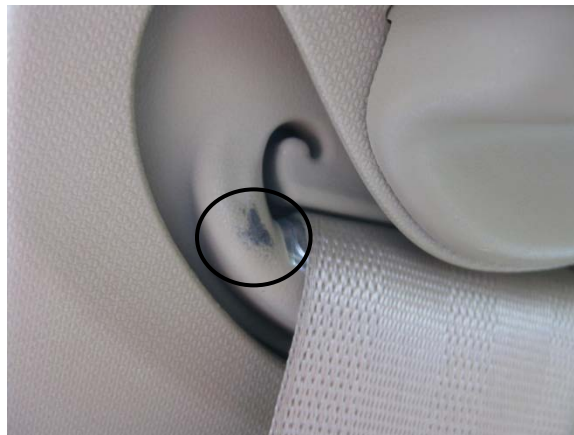
Figure 5. Grime and Wear caused by Normal Belt Usage (No Collision- Right Front Passenger)
