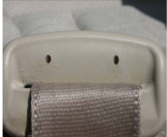
Figure 4. Damage to the Latch Plate after a Crash
