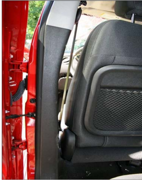
Figure 10. Bow String Effect caused by Pretensioner when Seat Belt was Unworn
