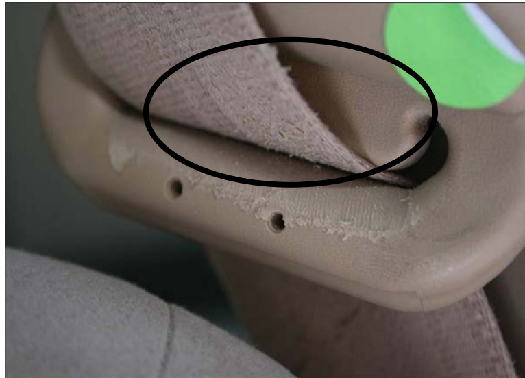
Figure 9. Friction Melted Plastic Transfer from the D-ring to the Webbing
