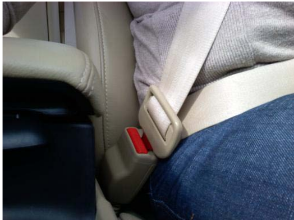
Figure 6. Directionality of the Seat Belt Webbing through the Latch Plate when Belt is Properly Worn
