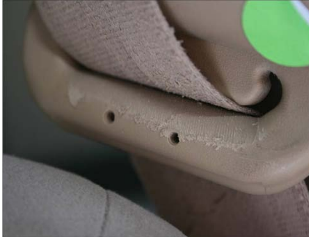
Figure 3. Damage to the D-ring after a Crash
