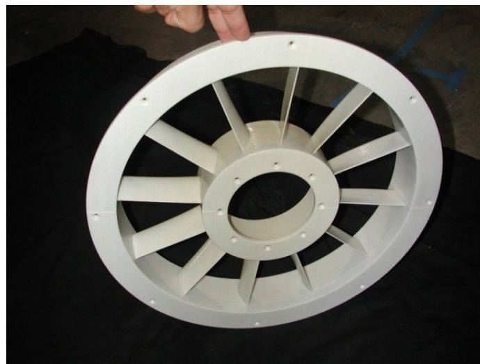
Figure 2–15: A perspective view shows the trailing edge of swirl vanes that induce the required swirl distribution
