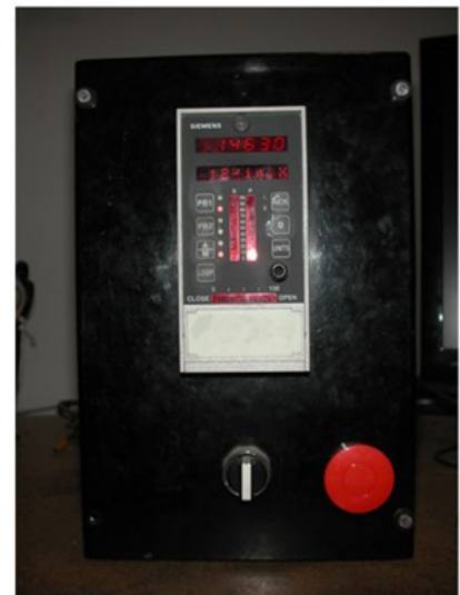
Figure 2–2: a) A short diffuser section connects the control valve to the pressurized tanks b) A Siemens controller was used to regulate the release of pressurized air from the storage tanks
