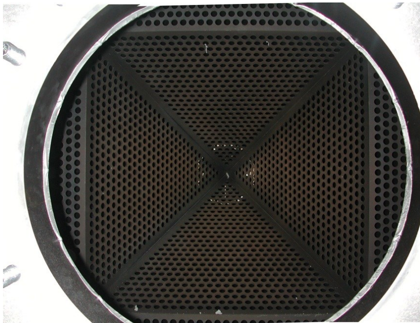
Figure 2-4: Looking upstream into the settling chamber towards the inlet of the expansion section, the geometry of flow spreader can be more clearly visualized
