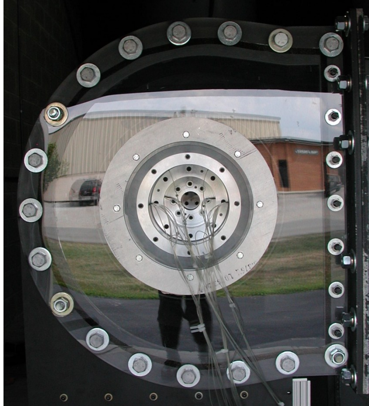
Figure A-7: Viewing access of the acrylic rear wall plate using the Techsburg facility orientation
