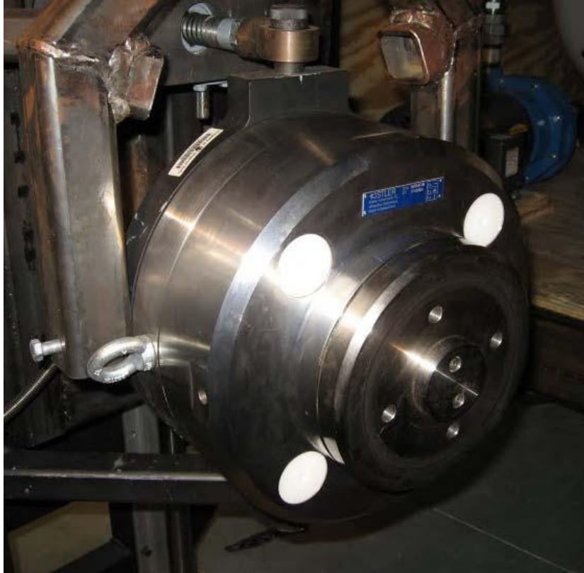
Figure 8. RoaDyn Kistler Force Hub Mounted in TTT. [Photo by author 2009]
