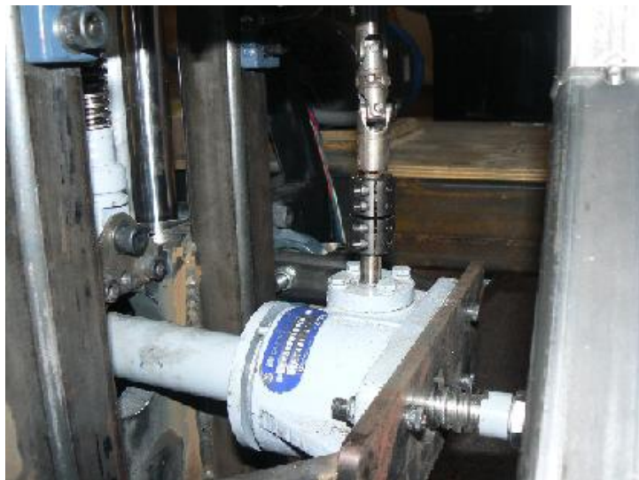
Figure 15. Steering Fork and Camber Mechanism Completed. [Photo by author 2009]
