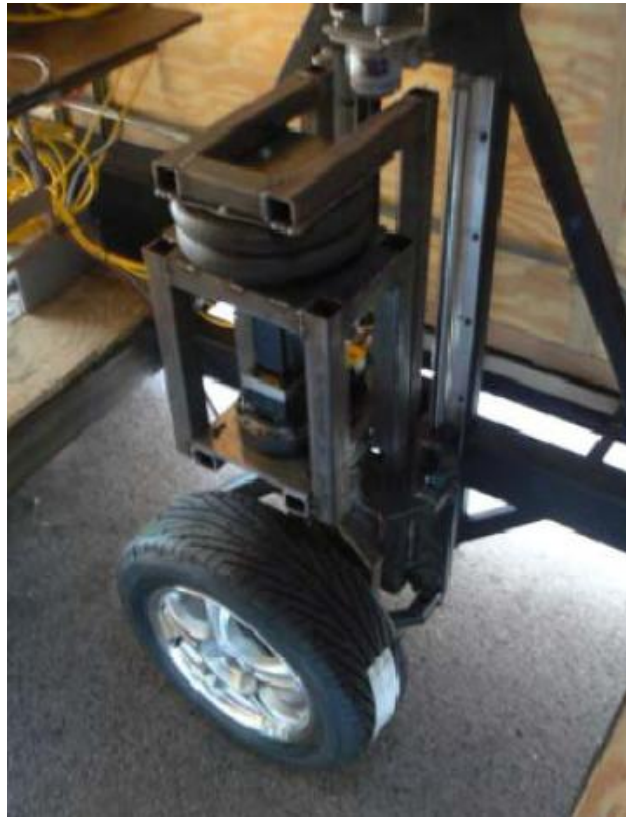
Figure 20. TTT Sliding Mounting Fixture With All Components Attached. [Photo by author 2009]
