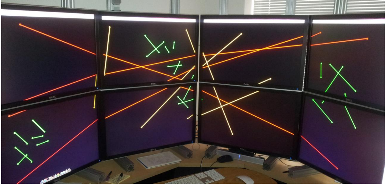
Figure 6: The screen used in the user study. Red, yellow and green lines demonstrate the concept of LMH technique in terms of distances covered with each multiplier. H is used for large distances (red lines), M is used for medium distances (yellow lines) and L is for short distances.
