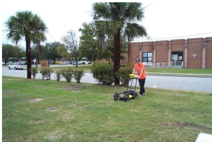
Figure 3-2 - GPR in Use at the USGS
