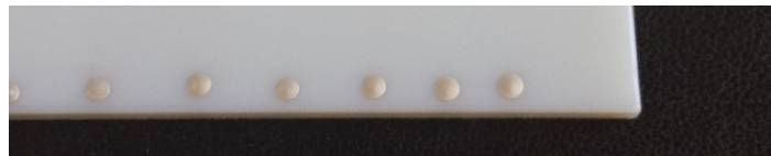
Figure 4.6: Droplets produced by 0.25 second dispensing pulses on VW substrate
