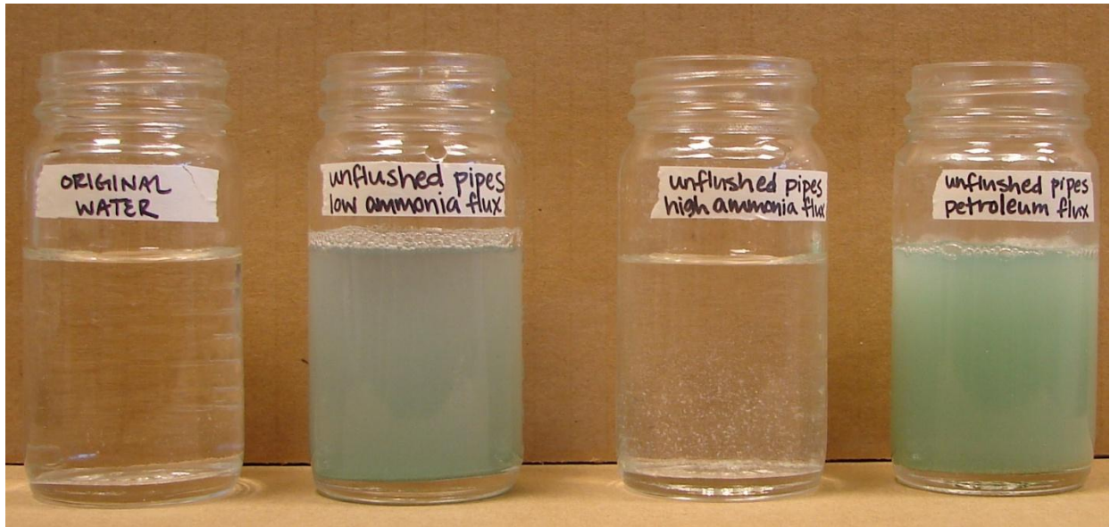
Figure 3-3. Visible effects of flux on water after an initial three week stagnation period in unflushed copper pipes.
