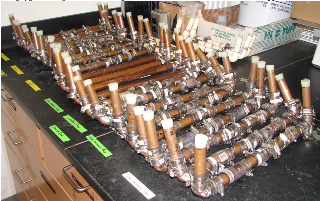
Figure 3-2. Complete set of pipes used in flux experiment.
