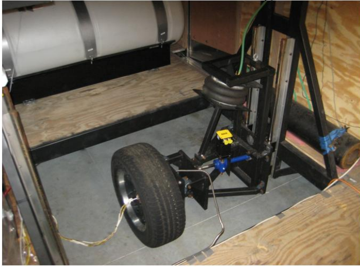
Fig. 2.9: Data for the dynamic tests collected using the in-house mobile tire test rig at the Intelligent Transportation Laboratory (ITL), Virginia Tech
