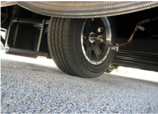
Fig. 2.10: (a) Instrumented tire prototype mounted on the test trailer, and (b) equipment housed in a trailer attached to a tow vehicle
