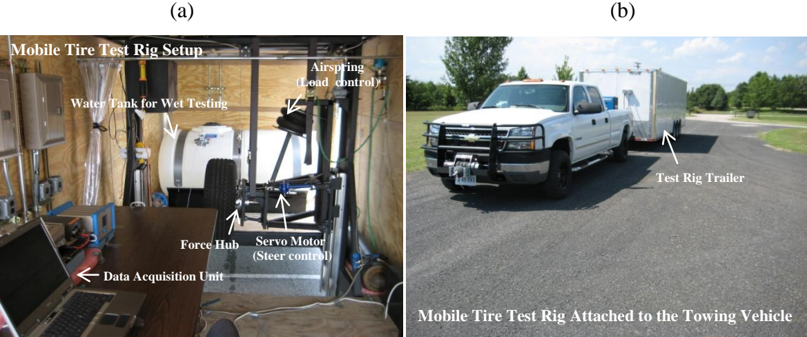
Fig. 6.13: Data for the dynamic tests collected using the in-house mobile tire test rig at the Intelligent Transportation Laboratory (ITL), Virginia Tech
