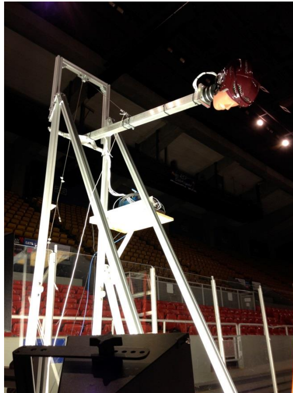
Figure 2. Pendulum set up on ice, in starting position for a frontal impact to the glass at a target velocity of 4.5 m/s. Photo by author.
