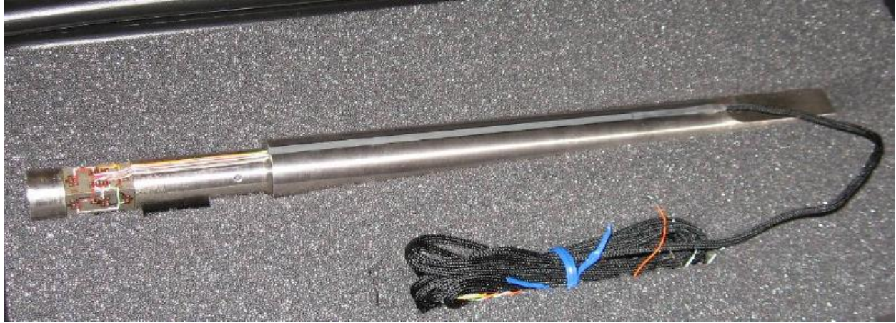
Figure 3.1. Three component strain gage force balance used to measure aerodynamic forces during wind tunnel testing.
