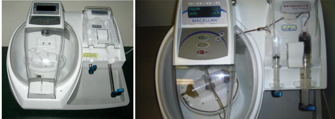
Figure 1.6 Magellan ® Platelet Separator System shown empty (left) and loaded with separation kit (right) (71, 73).
