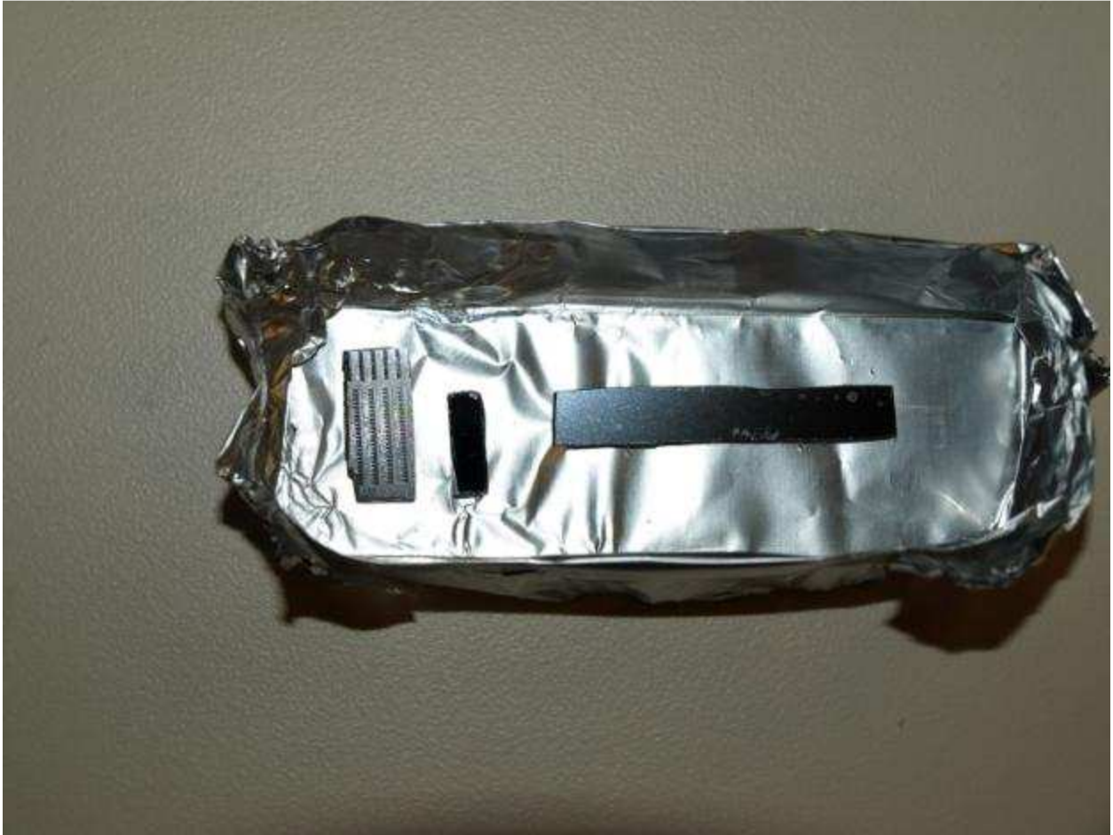
Figure 11: Silicon stamps covered in PDMS during the stamping process. Foil is used to create a mould, distribute heat, and prevent PDMS from leaking.
