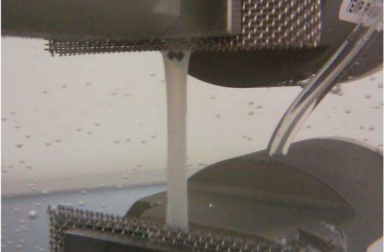
Figure 25: Failure of a cellulose network at the grippers under tensile load.
