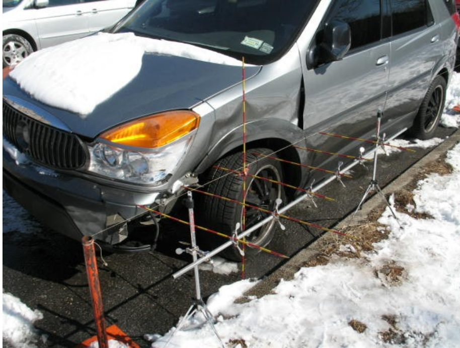
Figure 1. Measurement of a WinSMASH crush profile. NASS/CDS case 761011139, vehicle 1.
