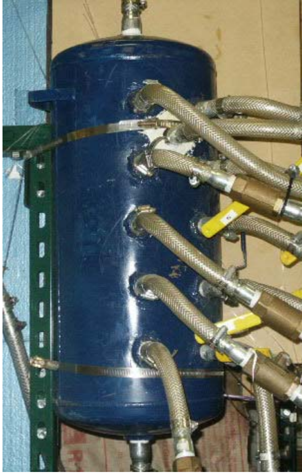
Figure 3-4. Octopus air tank used to control plenum feed flow. Air enters from above and below and exits evenly through the nine hoses.
