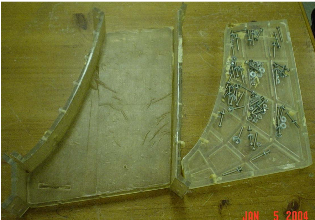
Figure 3.24 Pictures of the molds for the a) pressure side microcircuit and b) suction side microcircuit provided by Pratt & Whitney.
