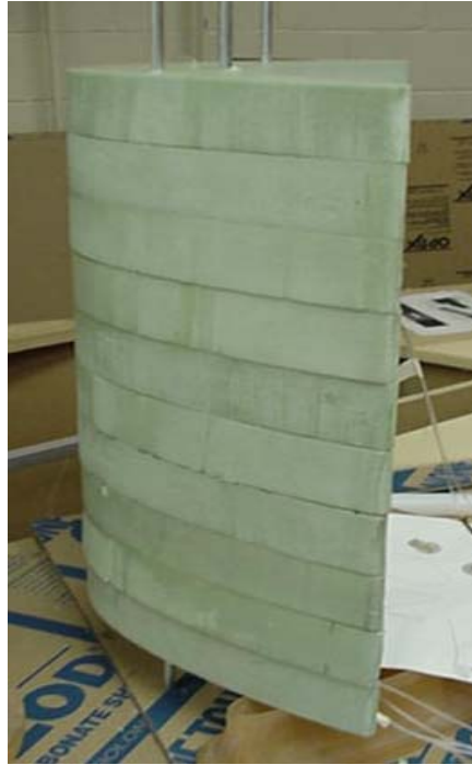
Figure 3.3 Picture of individual foam pieces as they are assembled into the final blade by using both glue and metal rods for strength.
