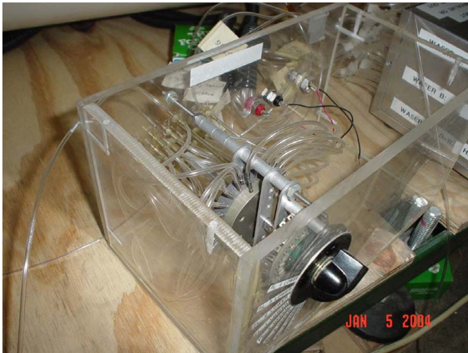
Figure 3.43 Picture of the pressure tap scanivalve wafer used to select one pressure to measure from 24 inputs.
