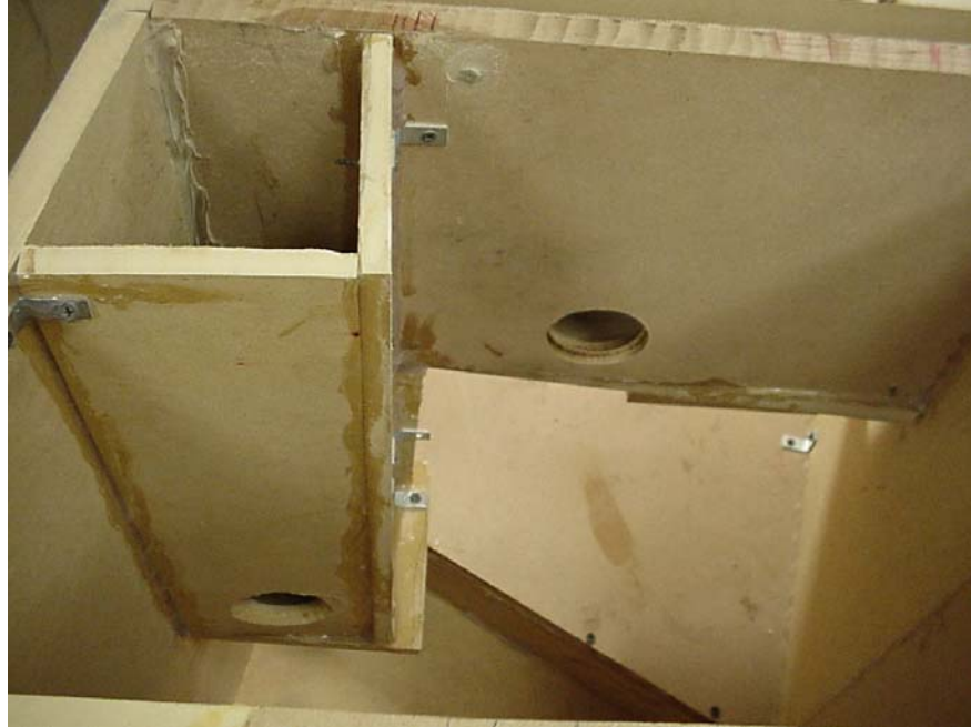
Figure 3.20 Side view of featherseal and suction side microcircuit plenum, showing 2” holes for the coolant flow through 2” PVC pipes.
