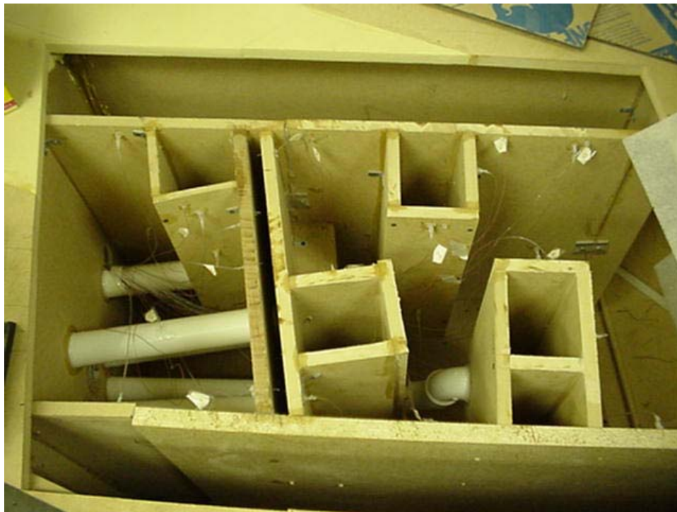
Figure 3.21 Picture of seven plenums after installing all the PVC piping, thermocouples and pressure taps.
