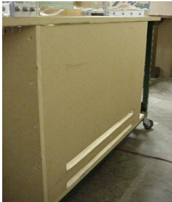
Figure 3.14 Picture of front of test section, showing the two slots that feed the front and aft rim plenums from the wind tunnel.
