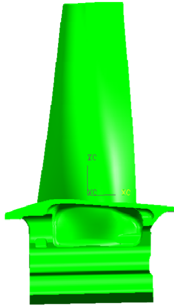
Figure 3.1 Side view of 1 st stage gas turbine blade showing the curvature of the hub region typical to most blades.
