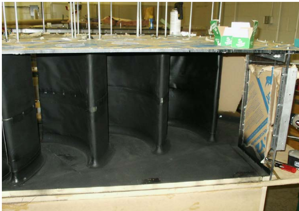
Figure 3.38 Picture the completed test section looking downstream from the combustor simulator exit, showing the three passage, four blade linear cascade.
