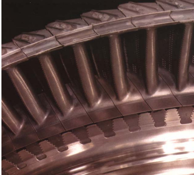
Figure 1.6 Picture of assembled turbine blade rig, showing the featherseal gap at the hub between blades. ( Gas Turbine Theory, 2001)
