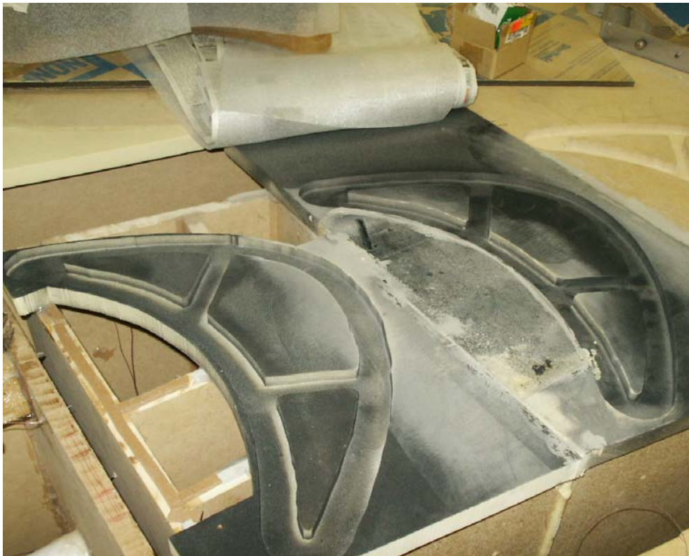
Figure 3.26 Picture of platform during installation of molded microcircuits, one pressure side microcircuit has been installed and the area for the second is visible.
