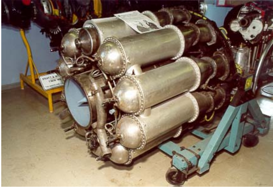
Figure 1.1 Picture of Whittle Engine test rig which successfully proved the feasibility of turbojet propulsion. ( http://www.visitcumbria.com )
