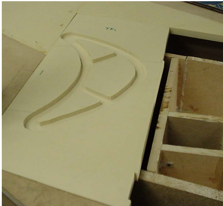
Figure 3.23 Picture of foam blade cut-out on top of the plenums, showing half of the feather seal gap, and the pressure side microcircuit plenum.
