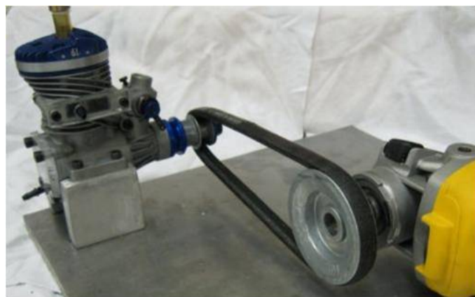
Fig. 4.4 Dynamics calibration mechanism for the fast-response probe
