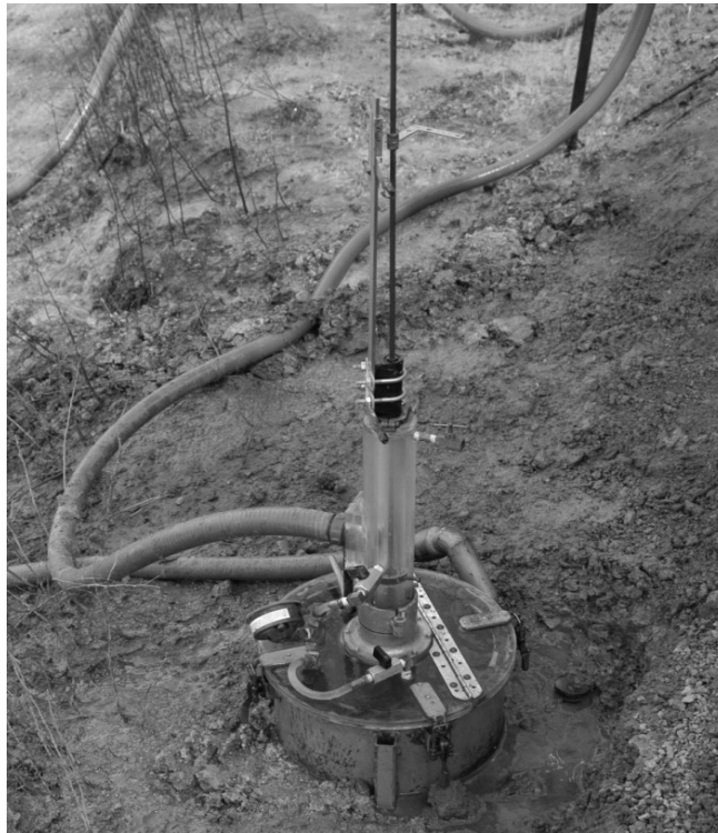
Figure 1 Jet erosion test device.
