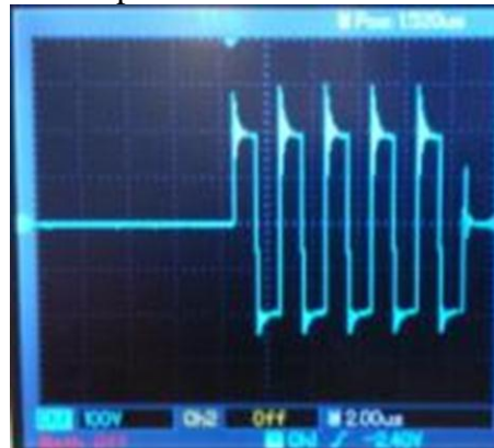
Figure 5-12: 200V peak (400V peak to peak) output waveform of the HFIRE electronics.
