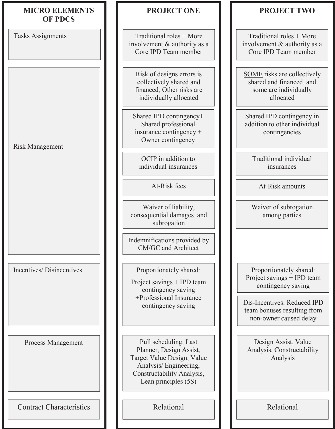
Figure 8-4: PDCS micro elements of IPD in “PROJECT ONE” and “PROJECT TWO”
