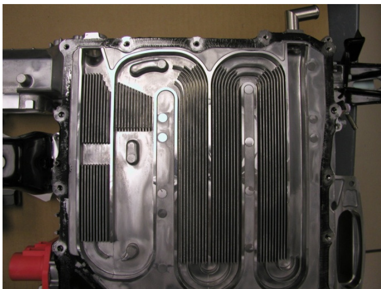
Figure 1.4. Typical heat exchanger used for cooling power control unit of hybrid vehicle.
