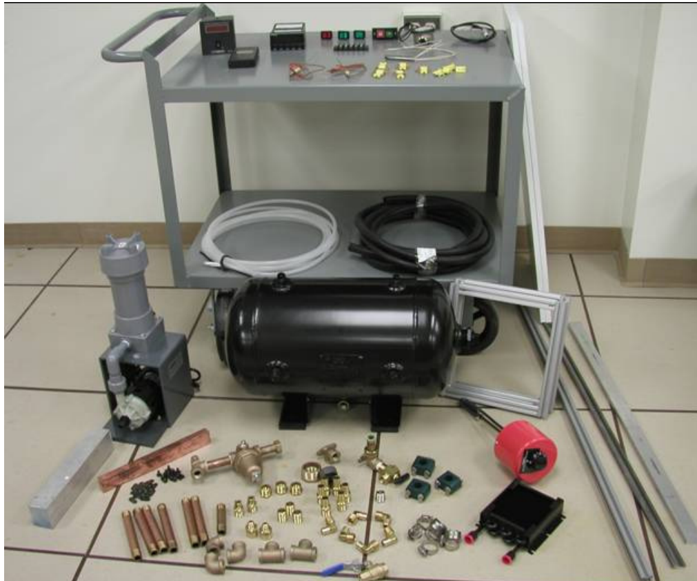
Figure 5.4. Various components of the thermal test bed before assembly.
