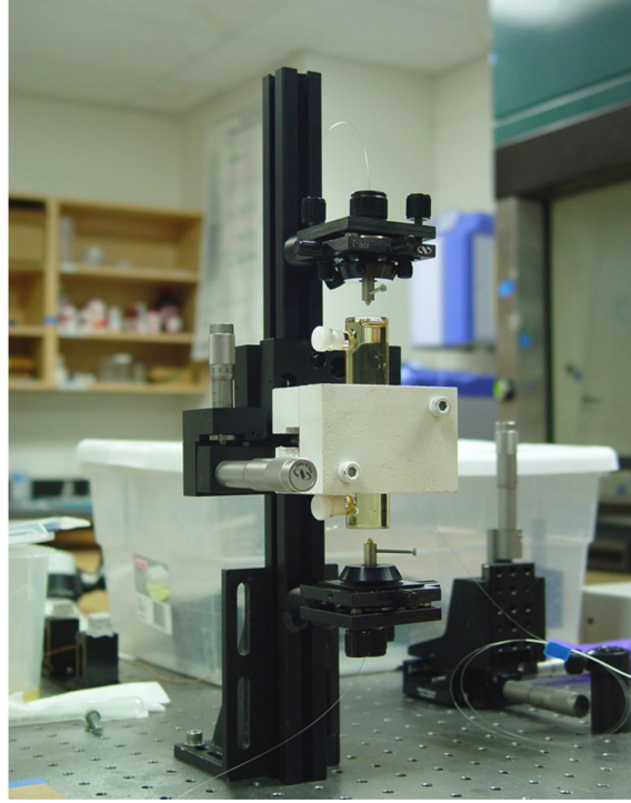
Figure 5-6: Acetylene detection system in vertical position.
