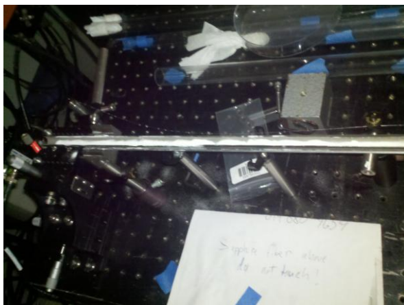
Figure 4.14 Alumina particle contamination of the single crystal sapphire rod housed inside half of a stainless steel tube
