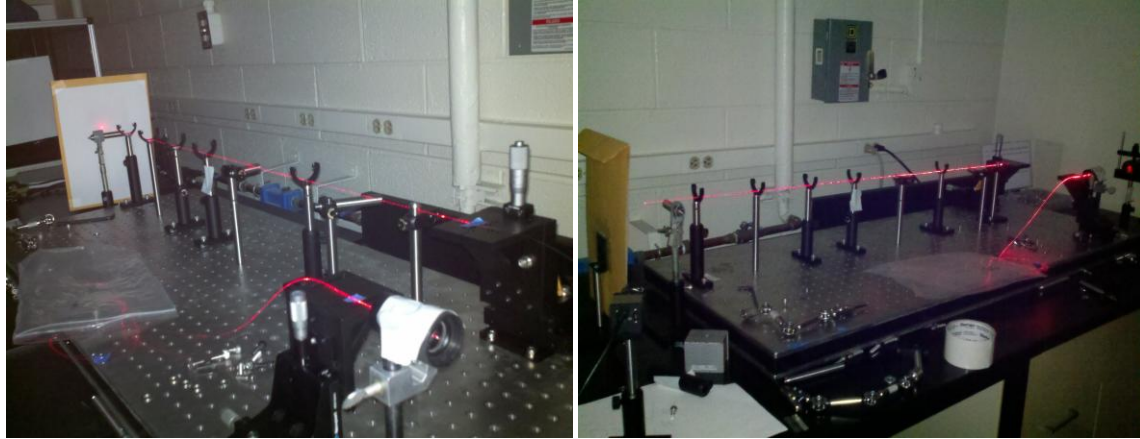
Figure 4.6 Far field imaging setup for all fibers tested
