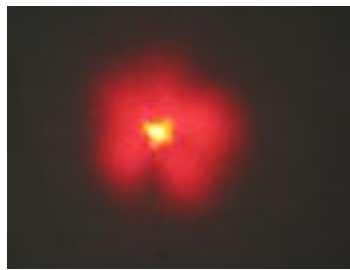
Figure 5.9 Far-field pattern for a meter length Corning SMF28 fiber
