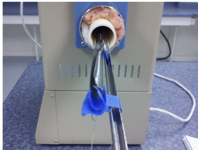
Figure 4.15 Single crystal sapphire rod and the 7-rod bundled single crystal sapphire fiber in their respective stainless steel tube housing in a horizontal tube furnace
