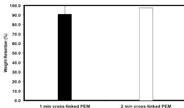
Figure 3.2 Retention in weight for cross-linked PEMs maintained at 37 °C and in PBS over a seven-day period.
