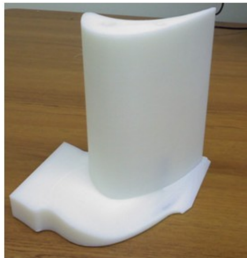
Rapid prototype model of airfoil A with contoured endwall
