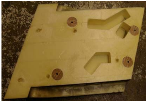
Figure C.9. Pack-H1 contoured endwall film cooling hole design and hole breakout pockets on underside of endwall.
