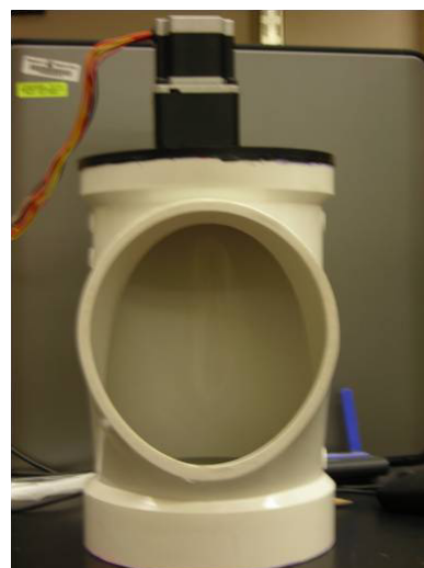
Figure 1.16 (right). Photo of PVC motor mount with stepper motor attached at top.
