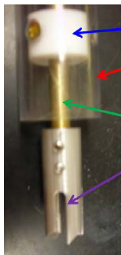
Figure 1.13. Photo of "claw" and driveshaft, showing (a) Teflon bushing, (b) plastic guard, (c) brass driveshaft, and (d) fluted aluminum "claw."
