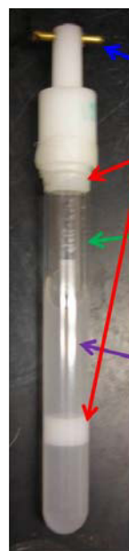
Figure 1.12. Photo of Couette cell, showing (a) brass crossbar, (b) Teflon spacers, (c) concentric glass NMR tubes, and (d) sample residing in sample gap.
