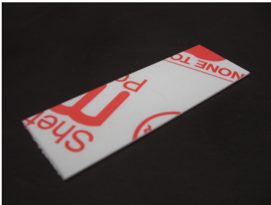
Figure 5.2 Makrolon ® GP Bisphenol A polycarbonate substrate cut to 1 X 3". The plastic masking has yet to be removed from the sample.
