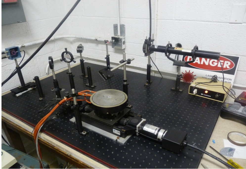
Figure 7-18. The optical setup for the curvature measurement [129] (Used under fair use guidelines, 2011).
