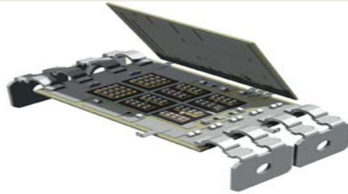
Figure 1-6. Power bump packaging for power module [26] (Used under fair use guidelines, 2011).
