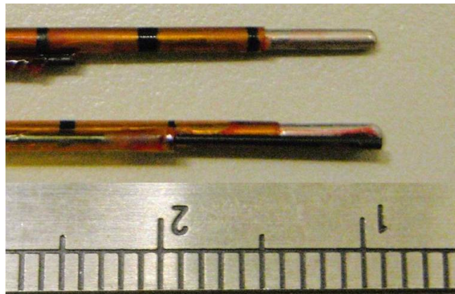
Figure 31: IRE electrodes used in the intracranial treatment of white matter with attached fiber optic probes to measure temperature during pulse delivery.
