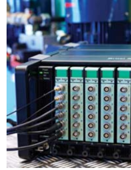
b) data acquisition modules for accelerometers
