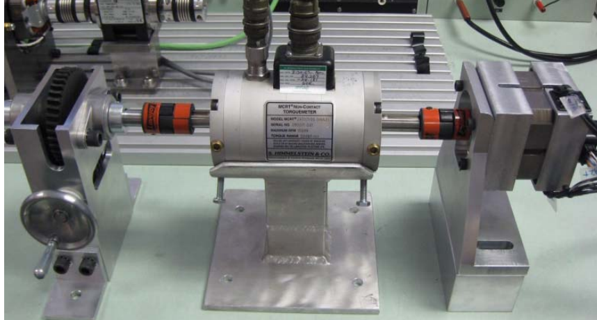
Fig. 5.23. Inductance and static torque measurement setup
