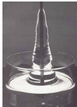
Figure 1.3: The Weissenberg or rod-climbing effect. The fluid is high-molecular weight PIB in low molecular weight polyisobutylene. Compare with water, where the swirling effect causes a depression rather than a climbing effect. From Boger and Walters (1993).
