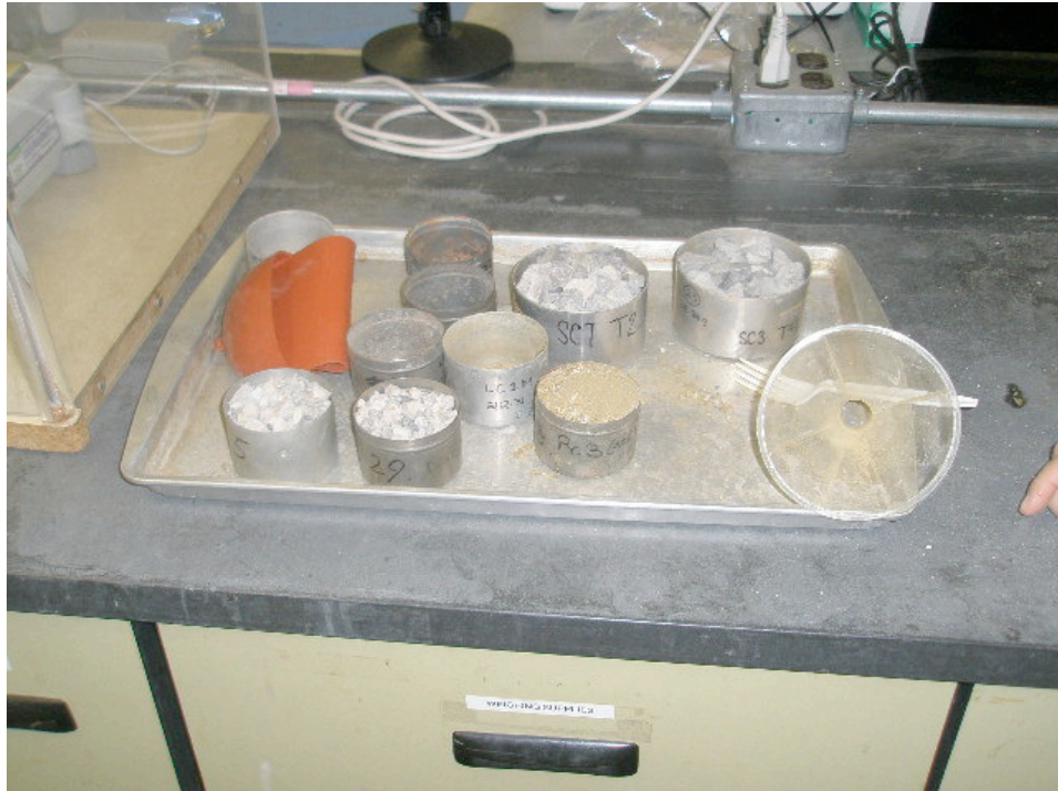
Bulk density testing on the various materials involved in this study
