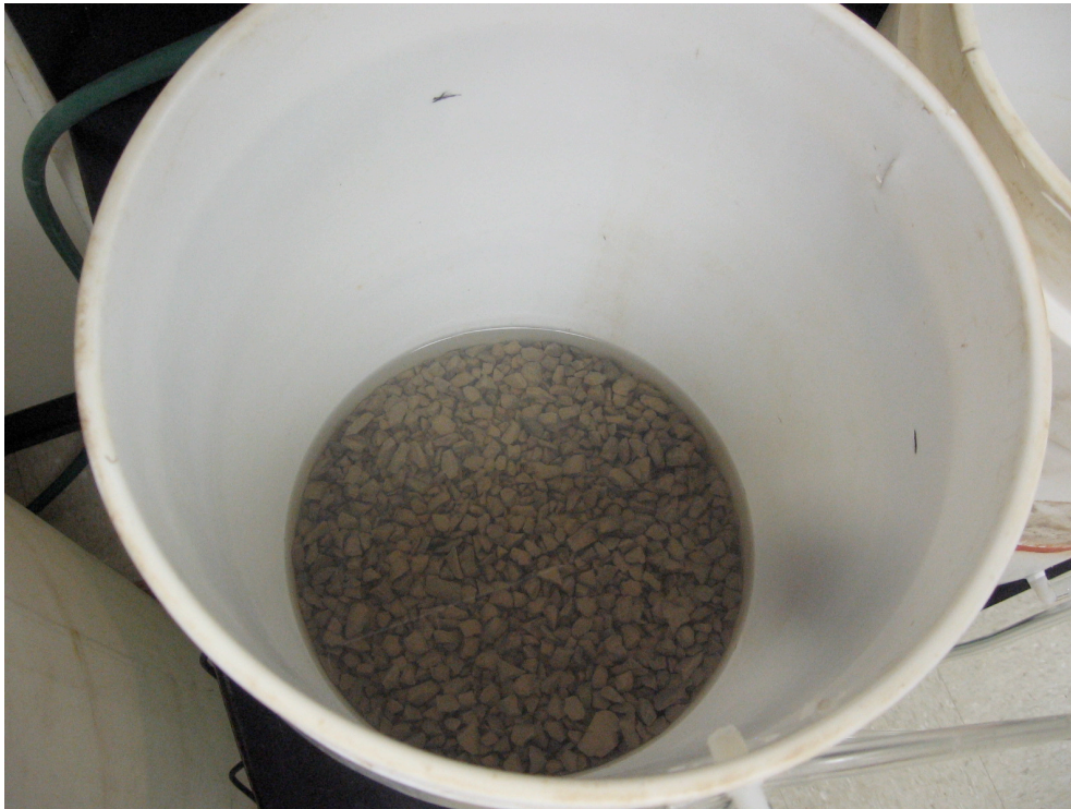
Gravel layer in the bottom of each experimental cell where the inlet was located
