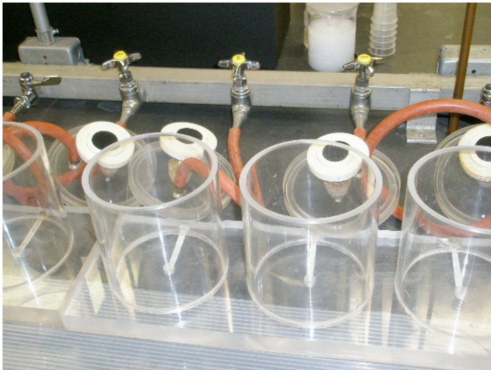
Filtration setup used for analysis of dissolved phosphorus
