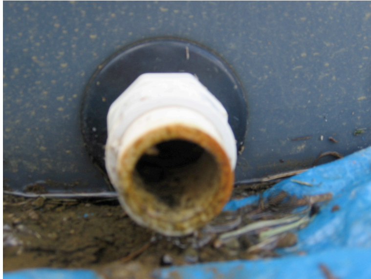
Fouling on water inlet after completion of the study
