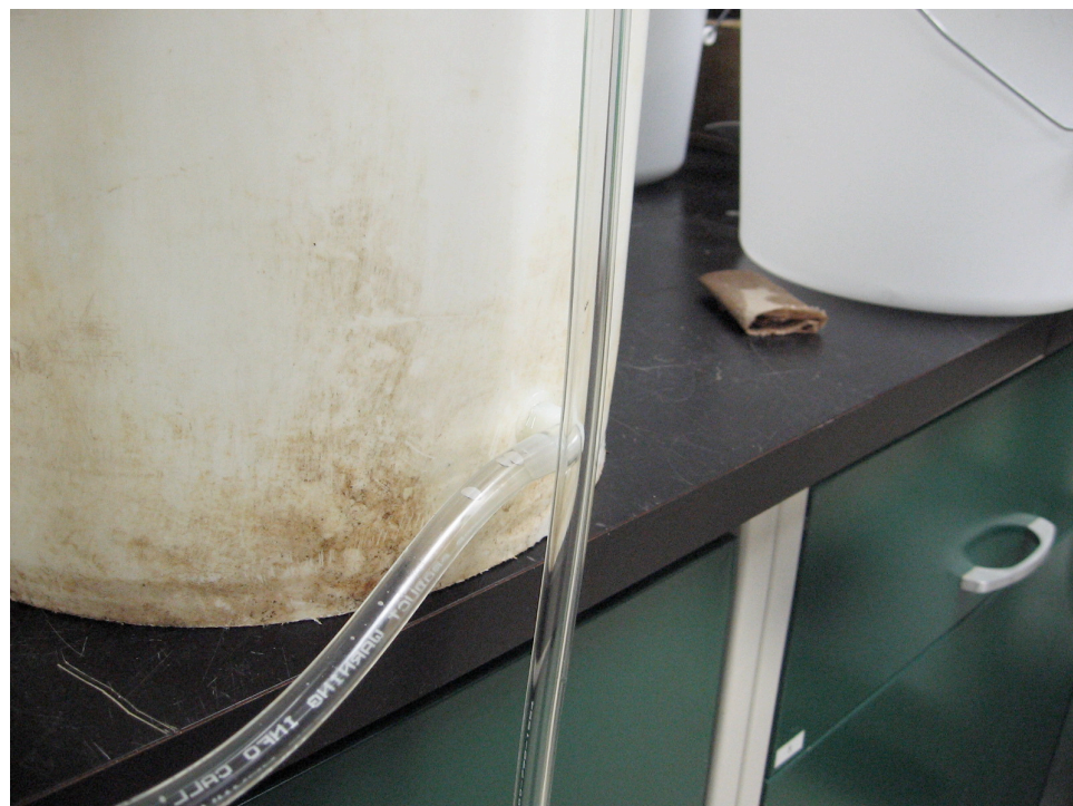
Fittings and tubing used to connect cells to the constant head tank and back to the holding tank
