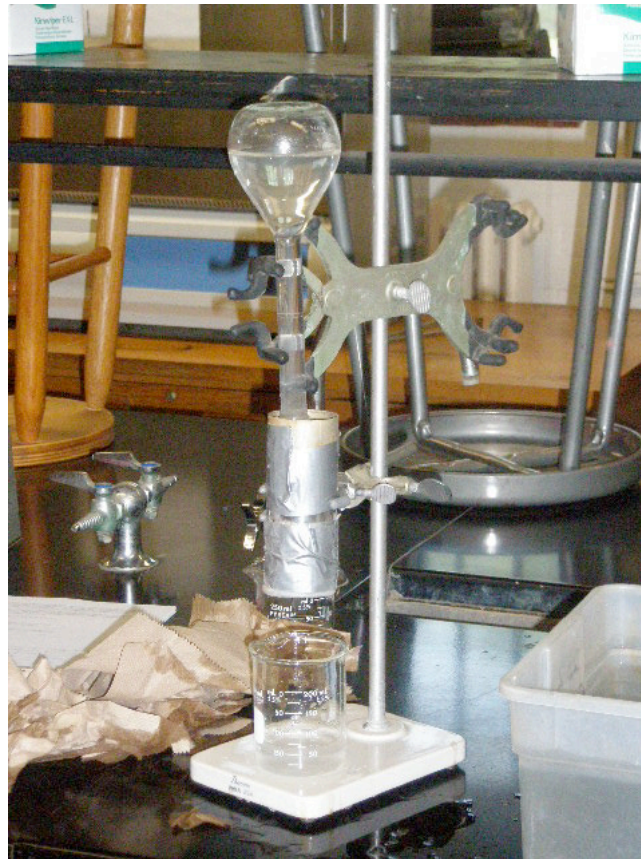
Experimental setup for hydraulic conductivity testing
