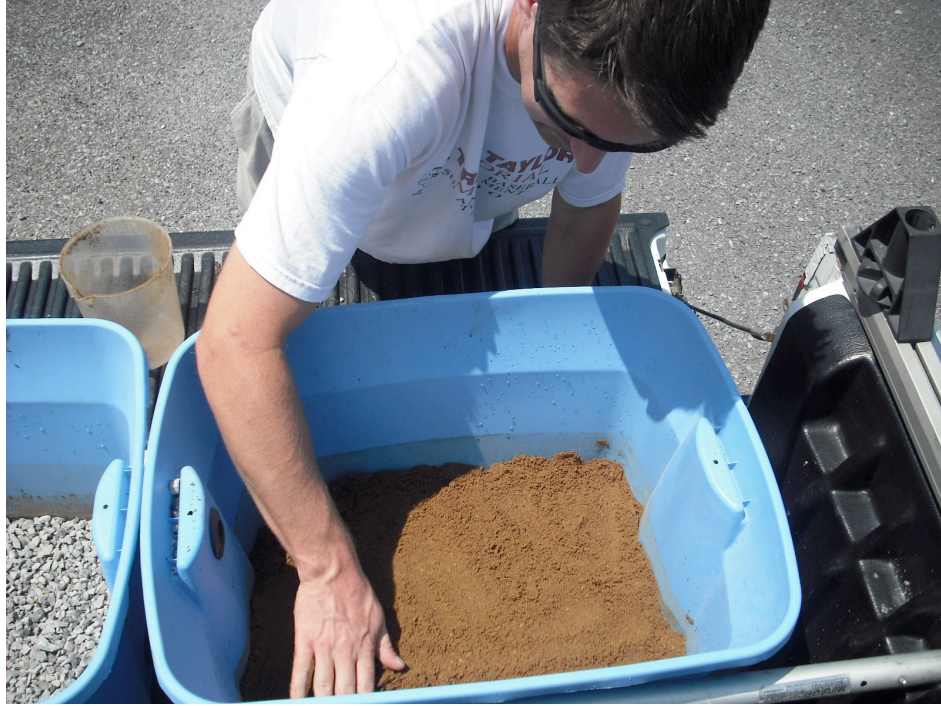
Finished filtration substrate layer
