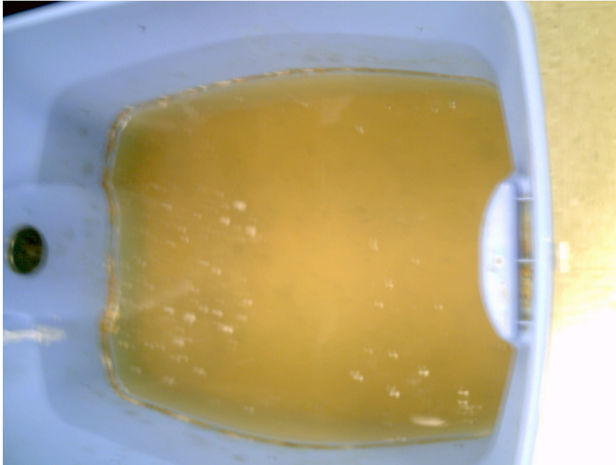
Sand-only cells produced little or no foam
