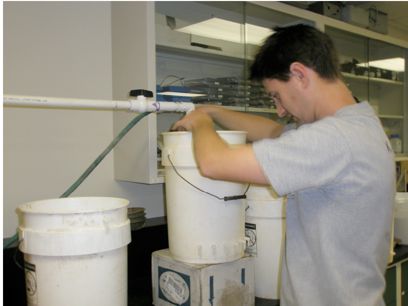
Constant head tank with associated plumbing
