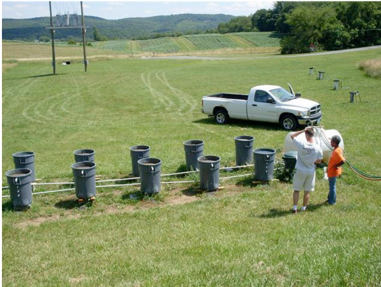
Experimental setup modified for follow-up study including raised concrete-block pedestals and head tank located below the pond with cells
