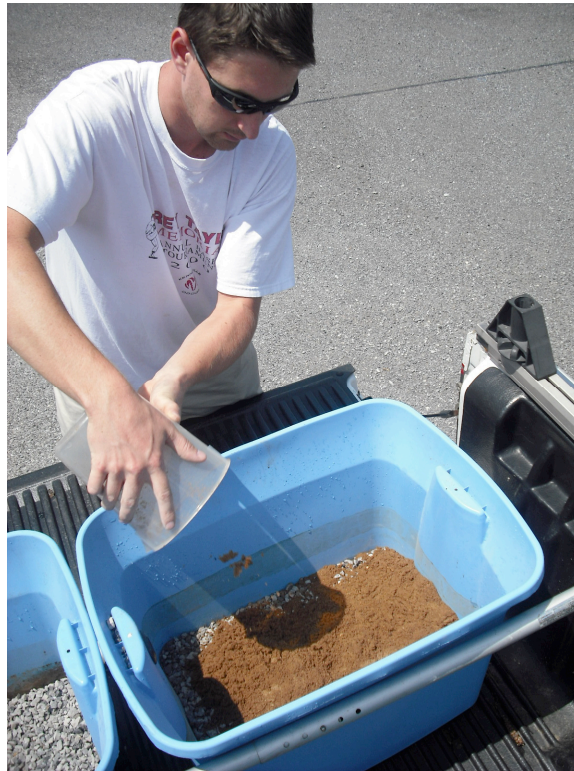
Adding the filtration substrate layer over the gravel layer
