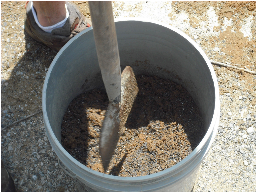
Mixing the Iron/sand substrate (1:2 volume ratio)
