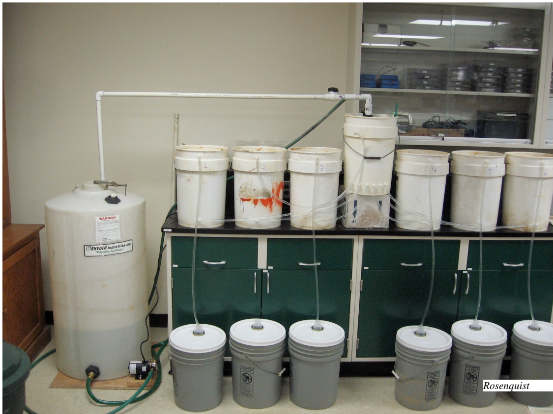
Completed setup being tested for flow rate before transitioning to single cell flow back to the holding tank including a view of the recirculation system which continuously mixed the tank water
