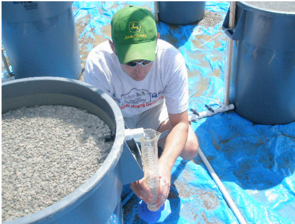
Taking a flow rate measurement on one of the experimental cells
