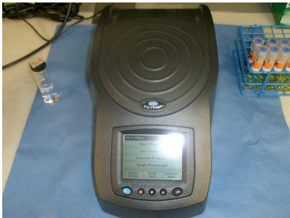
Photo spectrometer used for determination of phosphorus in samples
