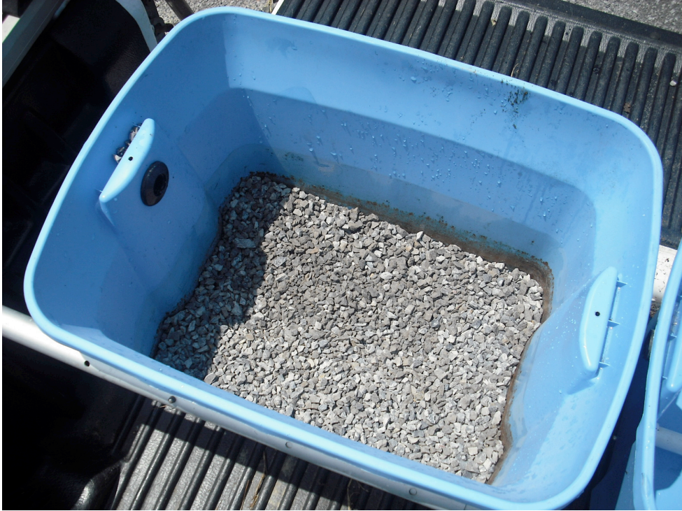
Complete bottom gravel layer with outlet structure covered
