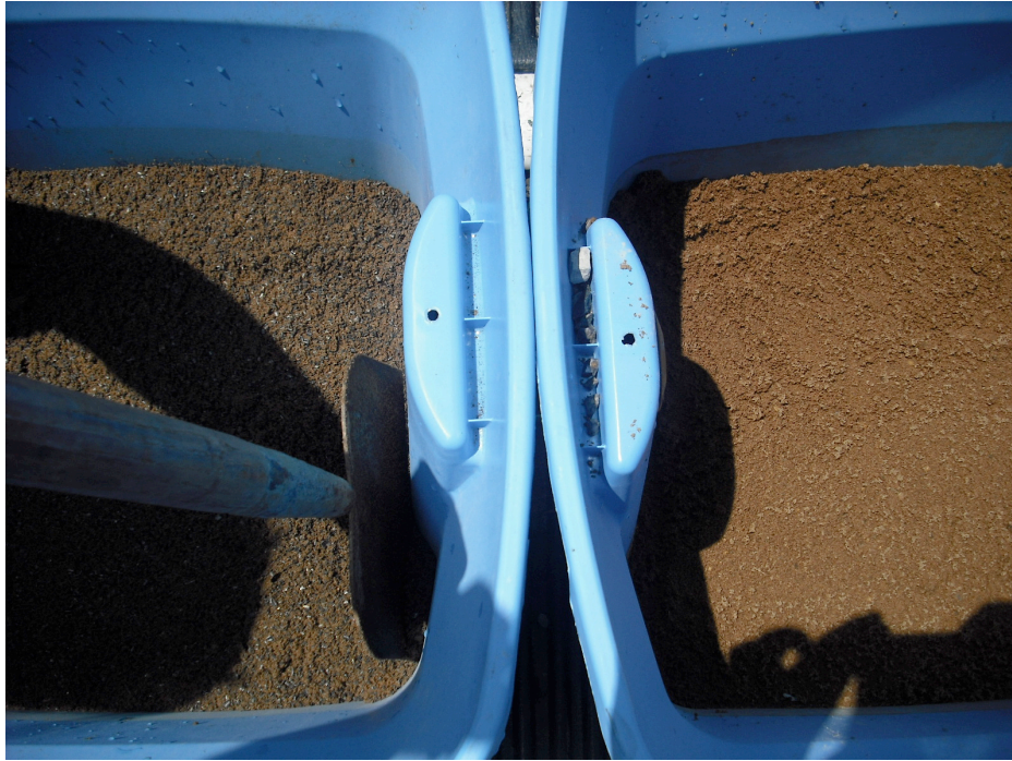
Iron/sand (left) and Sand-only (right) substrate layers in containers
