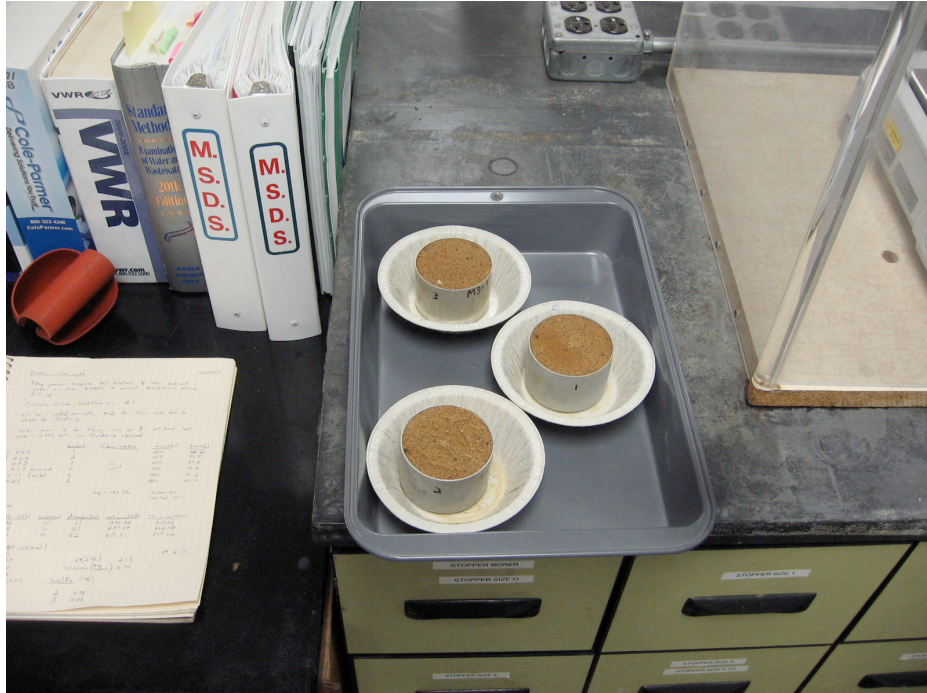
Bulk density testing on substrate
