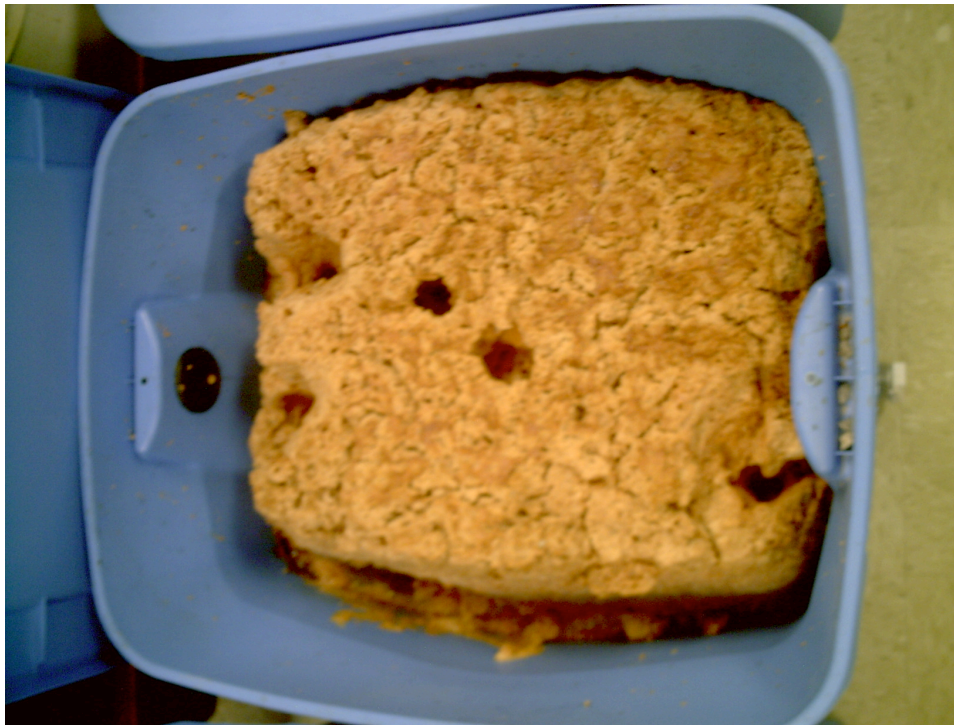
Foam present in iron/sand cells during rejuvenation
