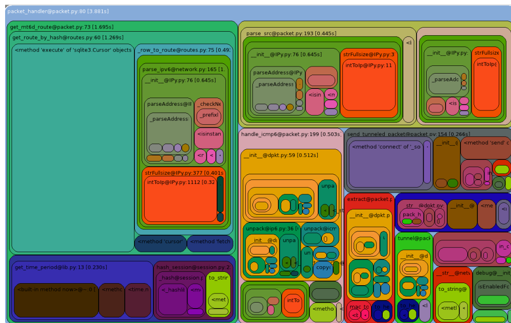
(b) Profile of the MT6D packet handler sub-process. Other components become visible when excluding libpcap from the code profile.
