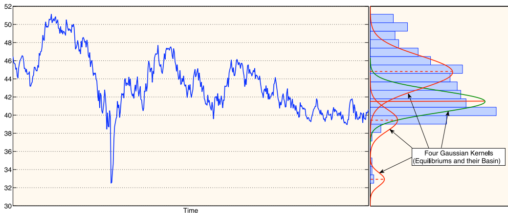
Figure 6-1: The trajectory and its nonlinear model with four equilibriums
