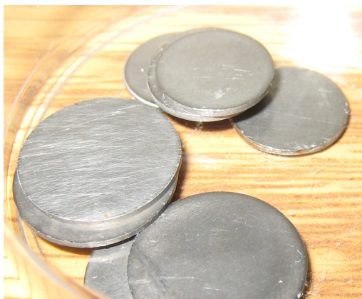
Fig. 6.1: Metal AFM pucks. Each puck has a 1 cm diameter.
