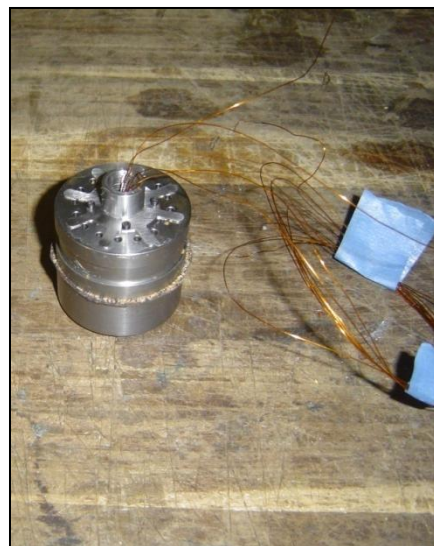
Figure 5-17 Assembled MR piston with gasket paper
