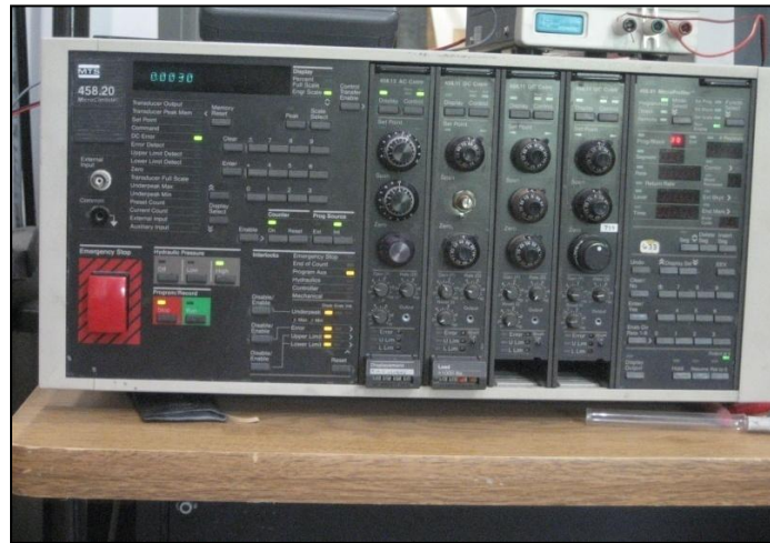
Figure 4-17 MTS 458 analog hydraulic controller
