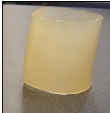
Figure 5-49 Polyurethane rubber made for use in MR pouches
