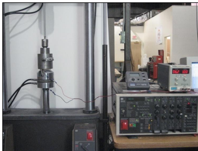
Figure 4-18 The rheometer installed in the load frame ready for testing
