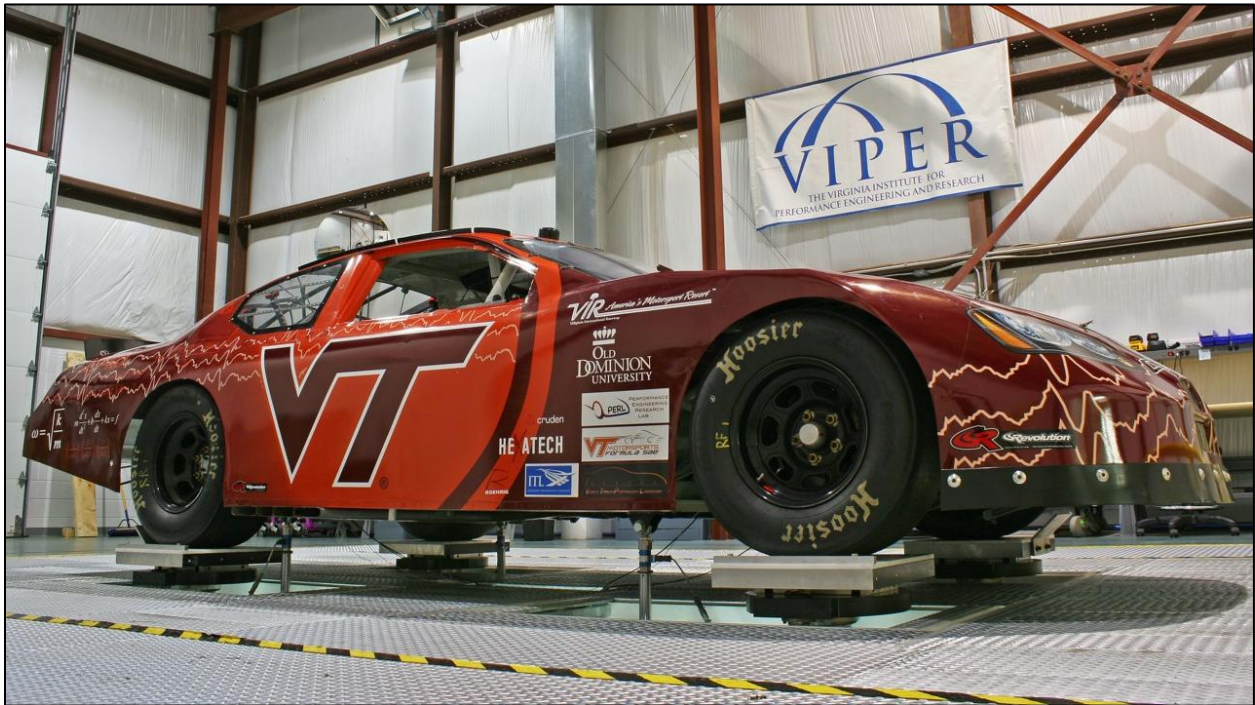
Figure 8-1 The 8-post shaker rig and the VT cupcar used to study suspension system performance at Virginia Tech. (CVeSS/VIPER test facilities)
