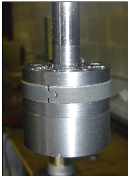
Figure 5-13 Assembled damper piston
