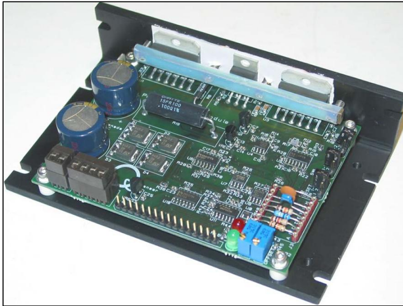
Figure 5-58 The linear current amplifier used to control the electric current passing through the rheometer coil
