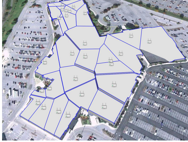
Figure 6.2: An example of an in-building deployment of our femto-cell layer. Polygons represent femto-cell coverage within a building. Locations of cHeNBs placement are indicated by the icons.
