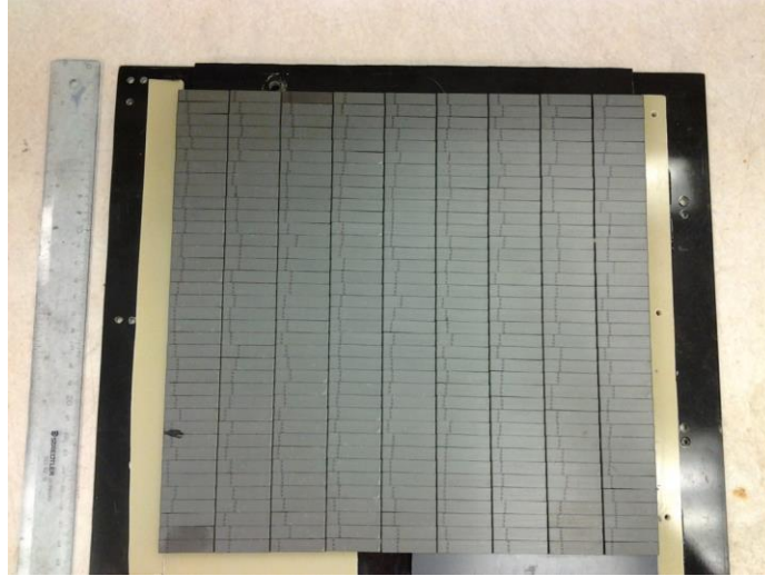
Figure 4.2 Ferrite Sheet Consisting of 9x37 Array of E-30 Size E-Cores
