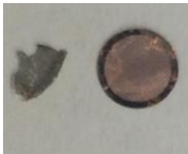
Figure S2. Extracted KTN film (left) formed on TEM grid (right).
