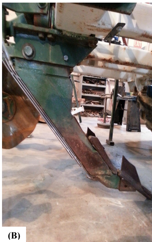
Fig 2.1a and 2.1b: Example of a strip-till implement and shank used for in-row subsoiling.
