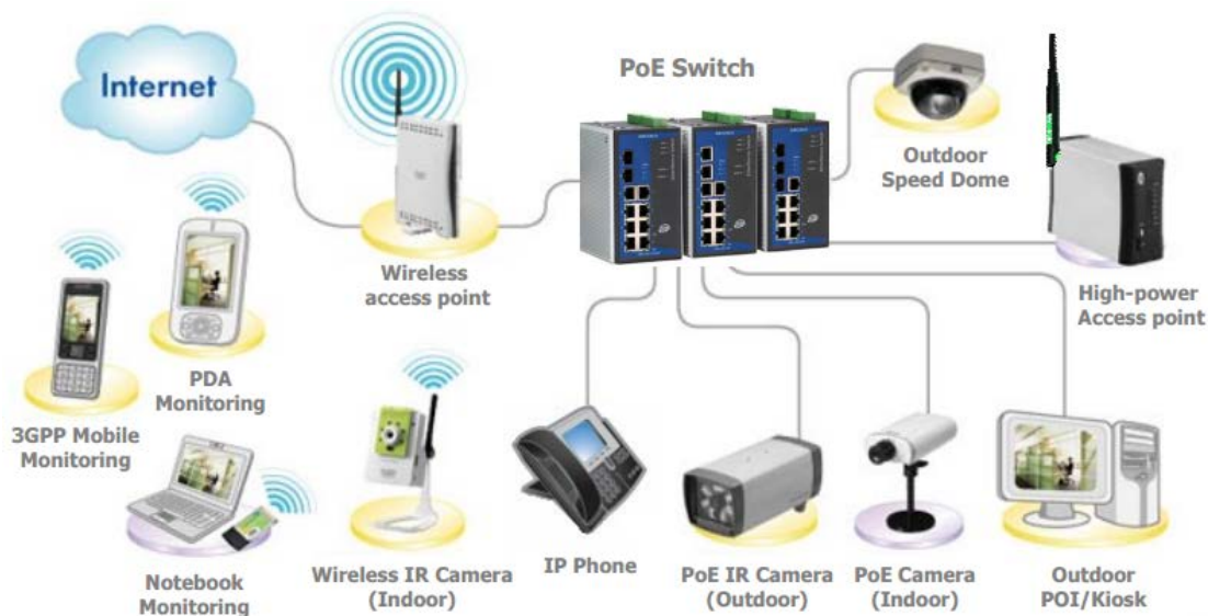
Figure 1.1. Power over Ethernet (PoE) system.
