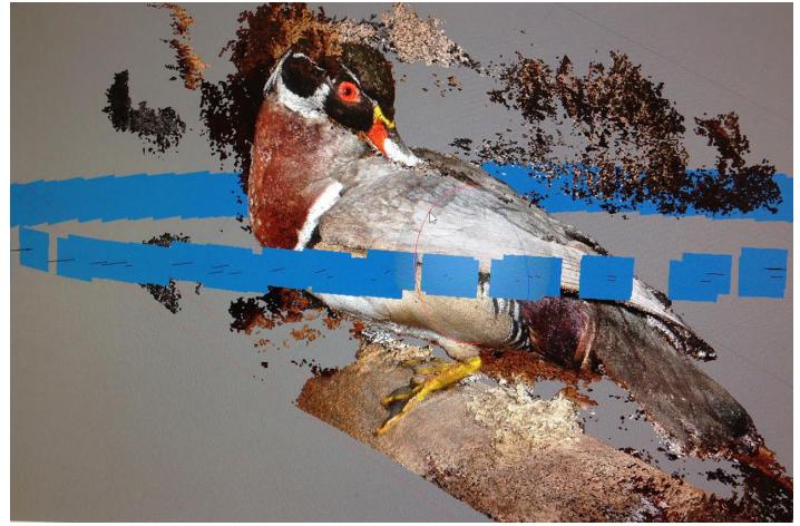
Figure 3.4: A completed wood duck model using Agisoft software. Each blue rectangle represents a photograph taken in relation to the original taxidermied animal
