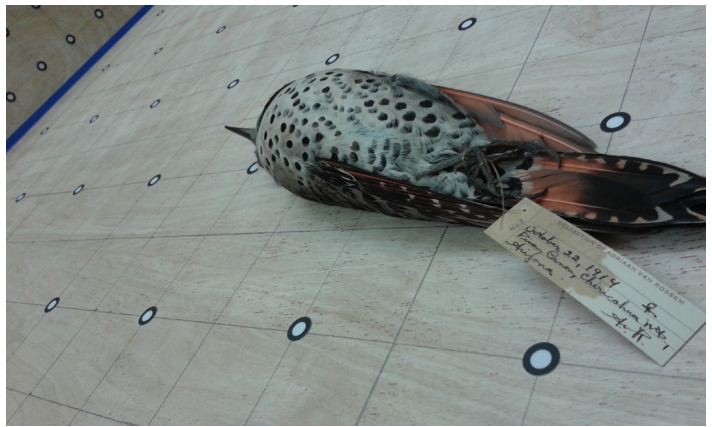
Figure 3.6: Northern flicker skin resting on scanning platform with locator dots
