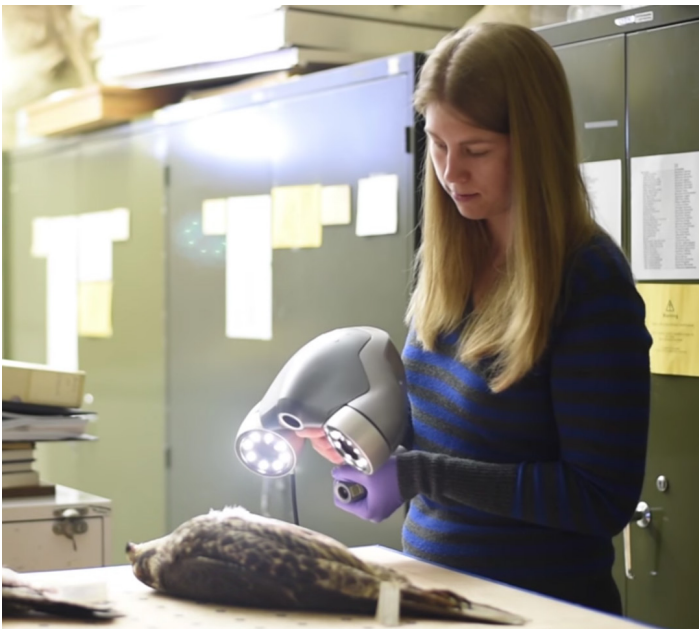
Figure 3.5: Using the Zcorp handheld scanner to scan a falcon
