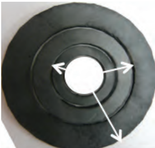
Fig. 3. (a) Three cells of inductor core made of ESL-40010 LTCC green tape. The height is 1.4mm and the radii from the innermost to the outermost cell are 7.6mm, 12mm and 18.9mm respectively. (b) Three-cell constant-flux inductor with core of 40.5 \times 40.5 \times 2.2 \text{ mm}^3 made of LTCC green tape with relative permeability of 41 and winding of flat copper (of thickness 70 \mu\text{m} ) having uniform distribution of flux density with B_{\text{max}} = 0.015 \text{ T}
