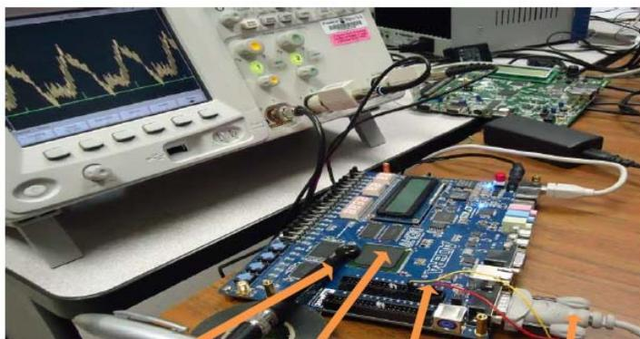
*Components of a side-channel analysis setup include an oscilloscope, and embedded board, and a control PC.*
