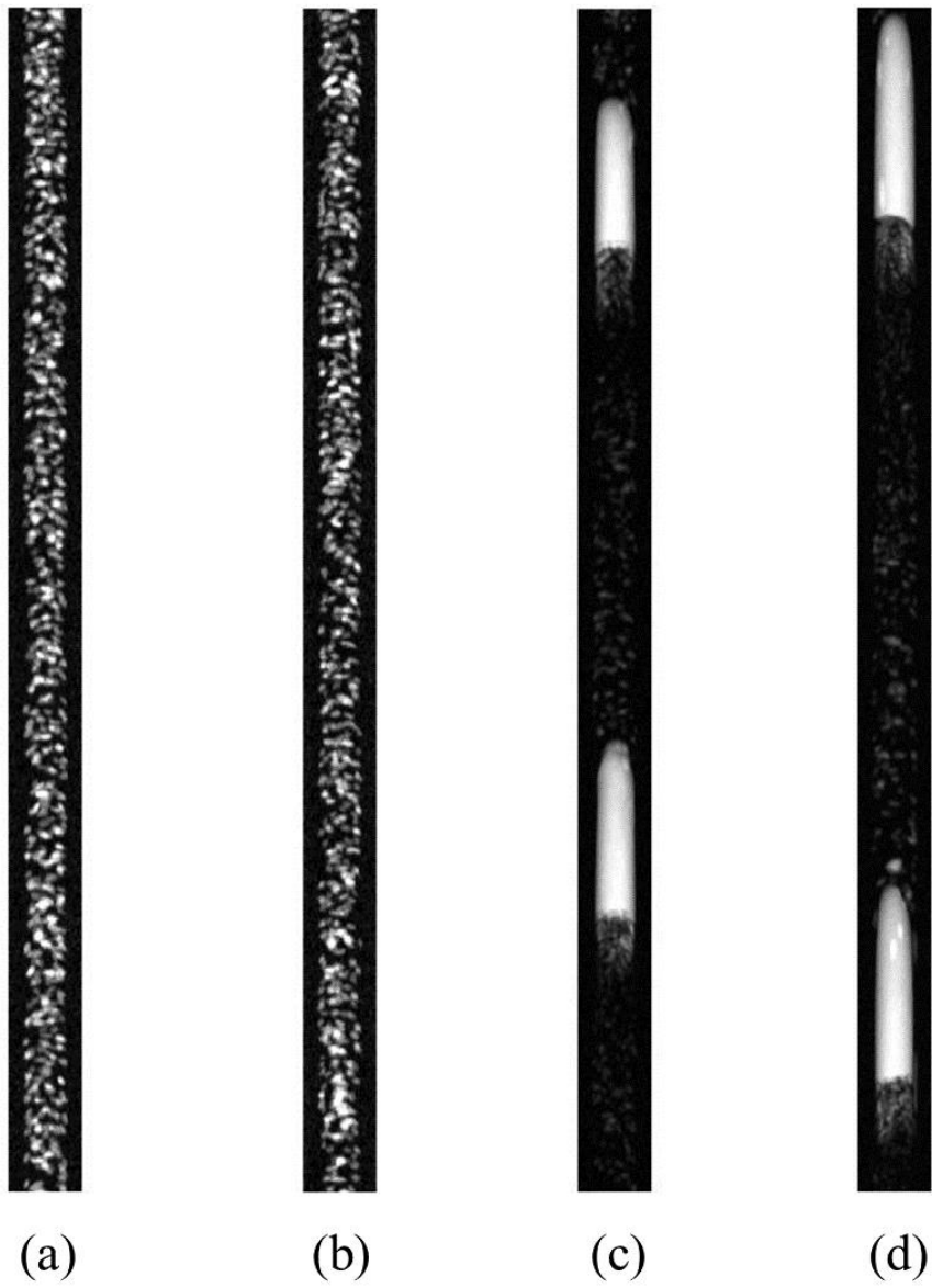
Figure 4-4: 2D reconstructed flow image from the bubbly flow (a) , (b) and the slug flow (c), (d).
